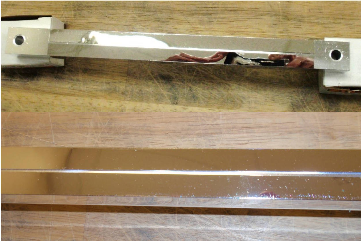
Pre-shaped ESR film on aluminum form (top); closer view (bottom)
